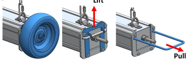
Grip the stainless-steel pull handle firmly and pull towards you. In the case where there is lots of debris collected, you may need to first pull swiftly to get the sleeve started off the magnet housing. It should get easier the further you pull the sleeve off.
