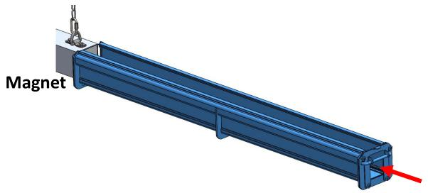
Place the black steel end cap on the other side of the sleeve assembly once the sleeve is pushed fully on. This end cap needs to be on the assembly to keep the sleeve on the magnet when sweeping for metal debris.
