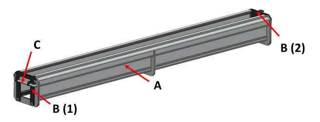
2. Remove B (2) from the sleeve. You only need to remove this end cap from the sleeve assembly before sliding the sleeve on your magnet (see next page)
